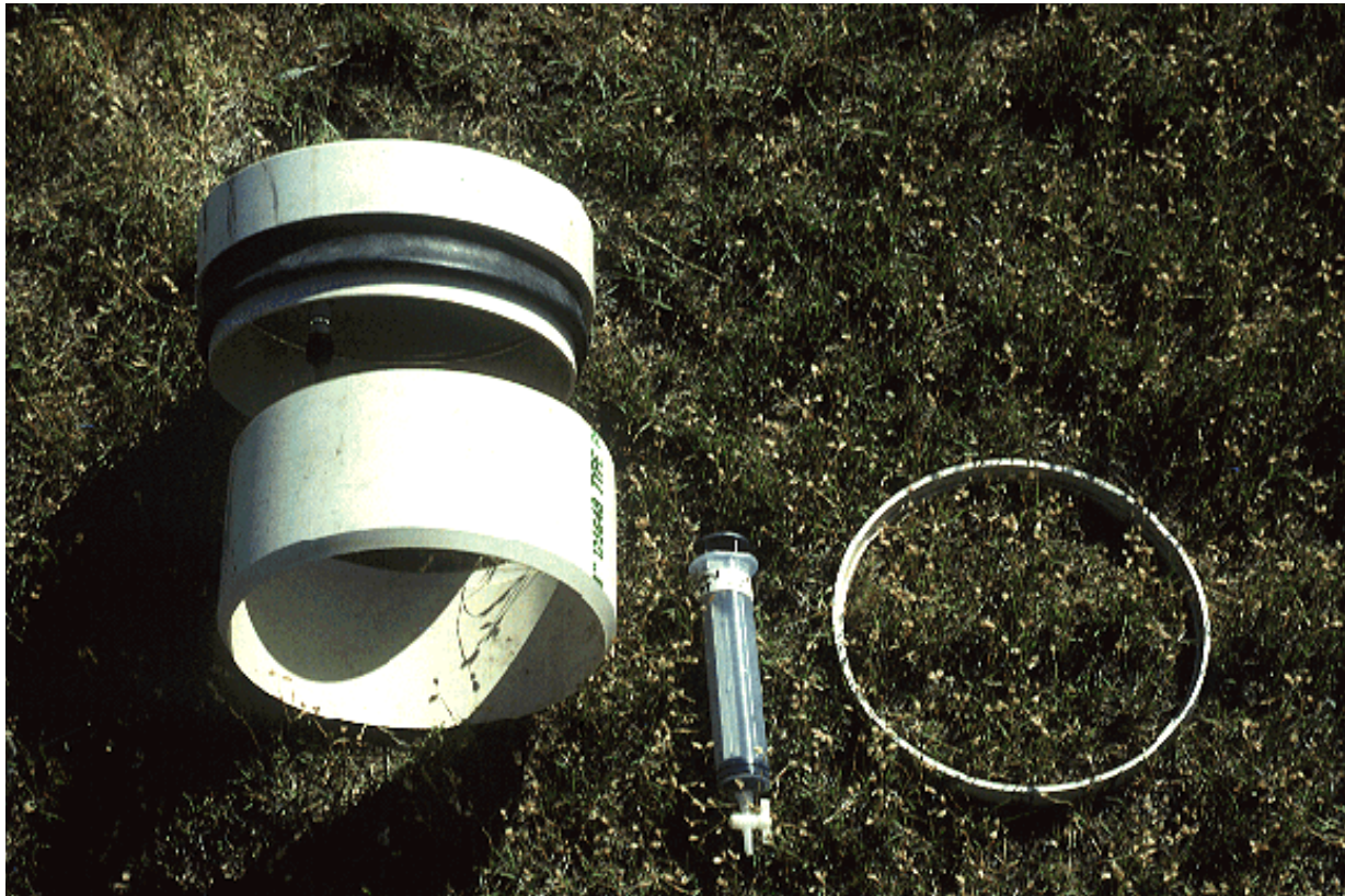
PVC soil anchor and chamber used by Hutchinson and Mosier.
