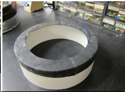
Fig. 6. Inner tube strip on PVC ring.
