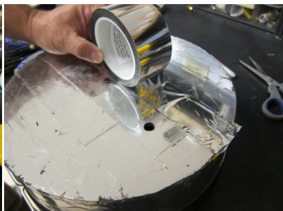
Fig. 21. Reflective mylar tape applied to chamber top.
