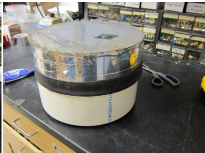
Fig. 25. Chamber on anchor – inner tube is folded up.
