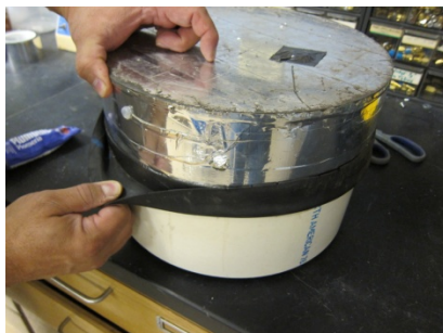
Fig. 26. Inner tube being folded down onto anchor.
