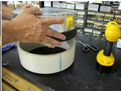
Fig. 25. Chamber is being placed on anchor ring.
