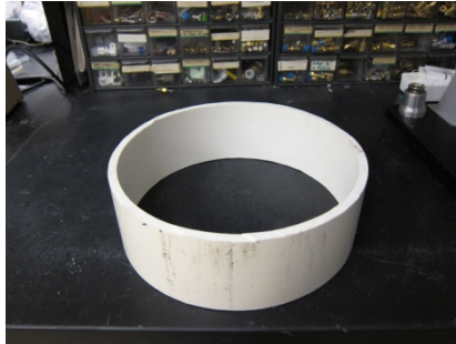
Fig. 1. PVC ring 30.3 cm inner diameter, 10 cm long.
