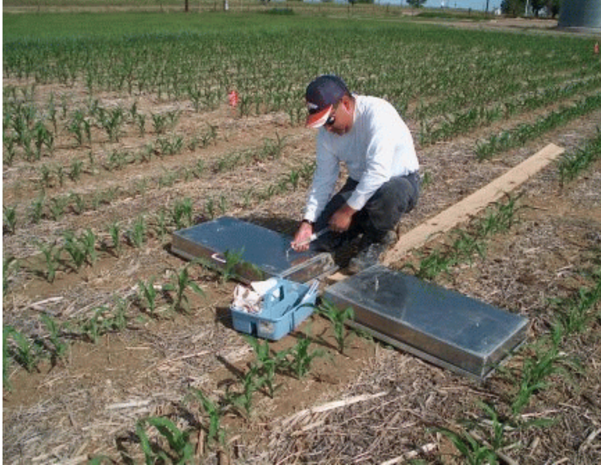
Rectangular Chambers used at Ft. Collins, CO Location.
