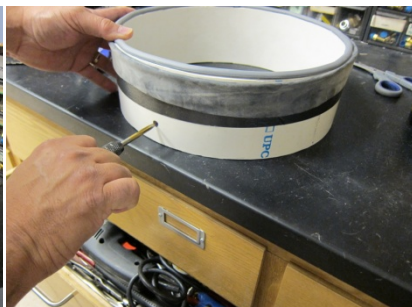
Fig. 15. Hole is tapped to accept vent tube fitting.
