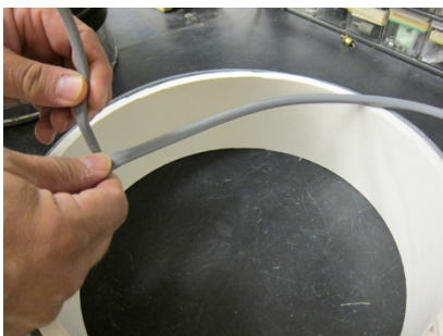
Fig. 11. Weather strip is first separated to single strand.
