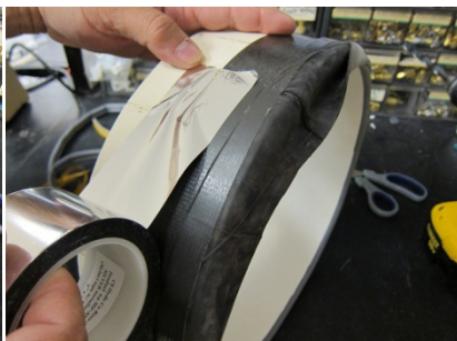
Fig. 20. Reflective mylar tape applied to chamber side.
