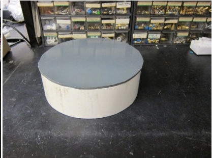
Fig. 3. PVC circle glued to PVC ring.
