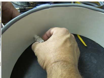
Fig. 17. Plastic union screwed into hole in chamber top.
