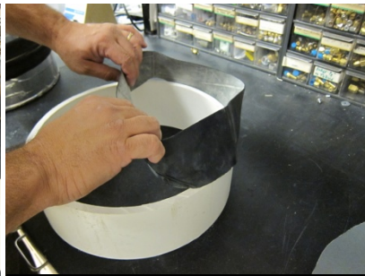
Fig. 5. Inner tube strip placed on PVC ring.
